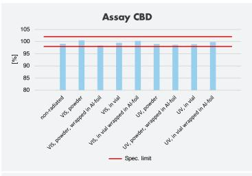
The CBD content lays within the specification limits of 98% to 102% for all irradiation variants (UV or VIS, powder or bottled, directly irradiated or packed in aluminium foil). No influence of light is noticeable.
